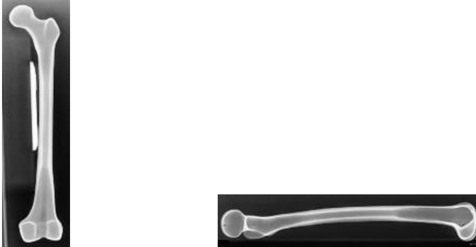
Figure 4-9 Digital radiographs of composite femur with size template (left - anteroposterior, right - lateral view)
