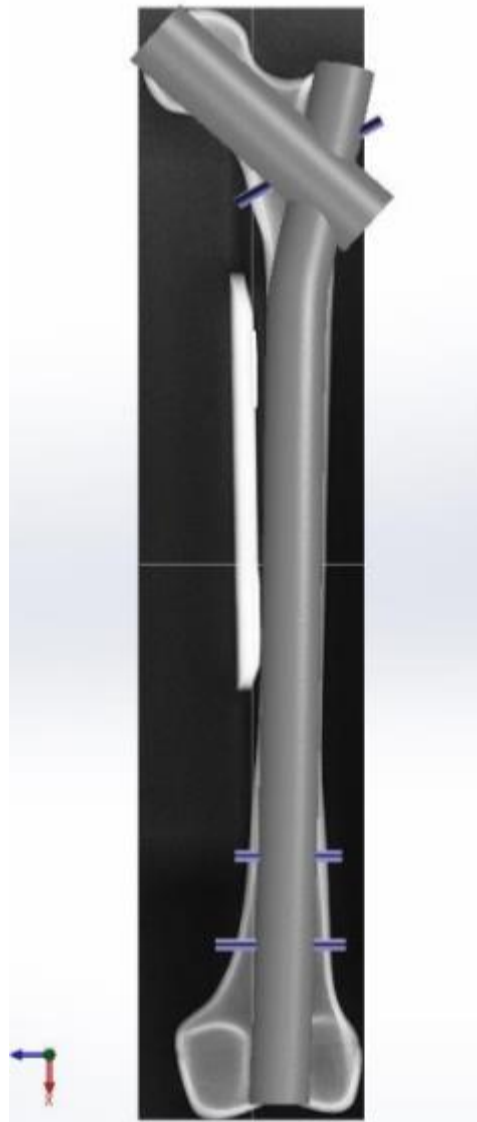
Figure 7-8 Final assembly of reamed femur, ALFN and interlocking screws representing paediatric femur fracture fixation FEA model
