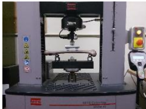
Figure B-5 Four-point bending test setup in the MTS machine showing top and base units
