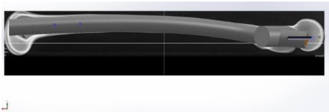
Figure 7-7 Creation of holes in the femur CAD model for the corresponding proximal and distal interlocking screws
