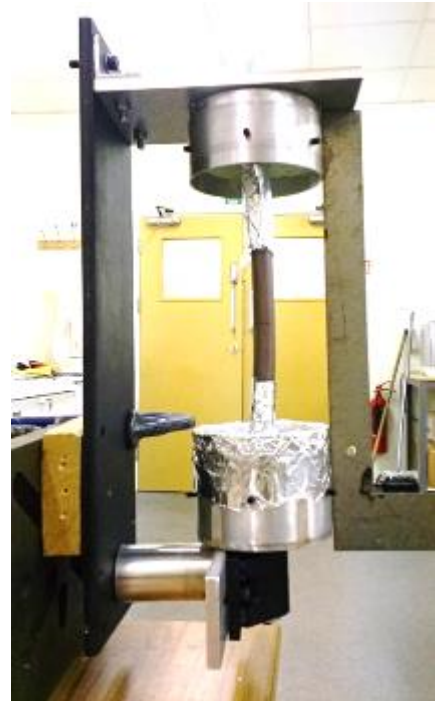
Figure B-8 Alignment of femur during casting of PMMA molds to ensure mechanical axis of femur was coincident with axis of rotation of the jig
