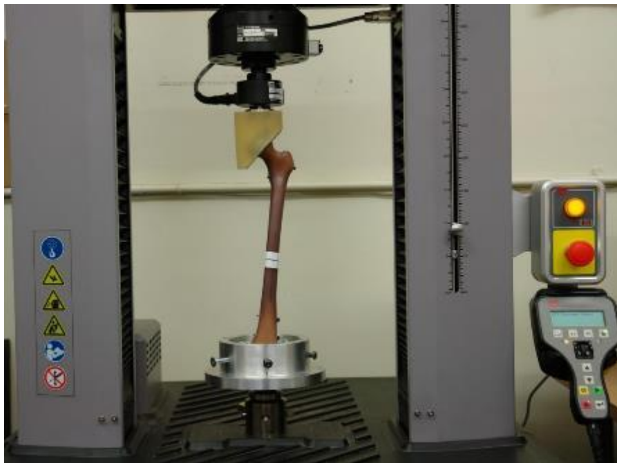
Figure 6-9 Axial compression test setup using the MTS testing machine showing the femur with a transverse fracture and ALFN in situ
