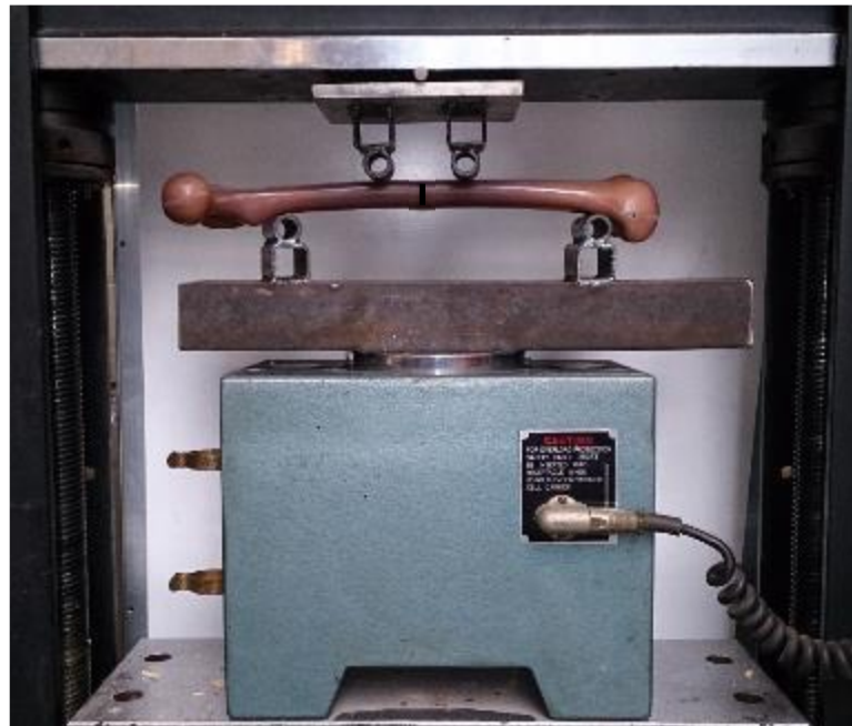
Figure 4-12 Four-point bending test setup
