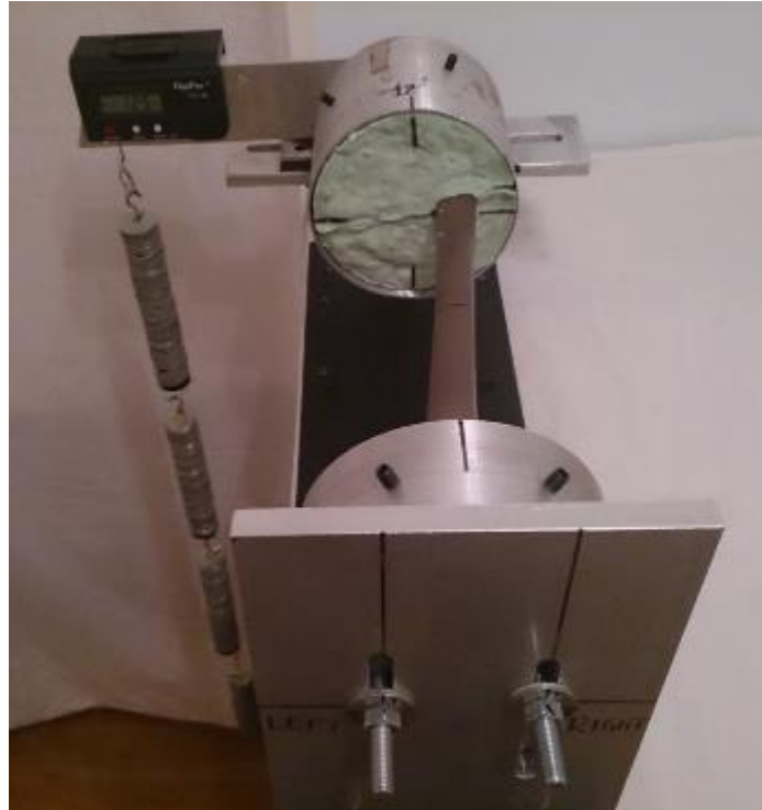
Figure 4-13 Torsional test (internal rotation) setup with calibrated weights
