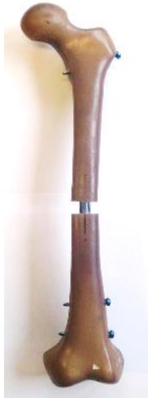
Figure 6-8 Simulated midshaft segmental defect with a fracture gap of 10 mm
