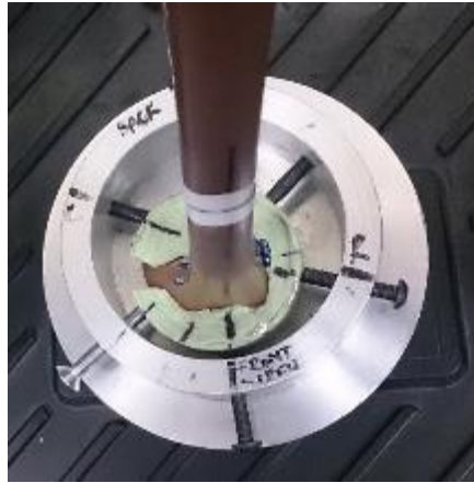
Figure B-1 Base unit with PMMA mold and screws securing distal end of femur
