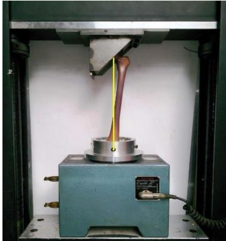
Figure 4-11 Intact femur aligned along mechanical axis in Instron materials testing machine during axial compression test
