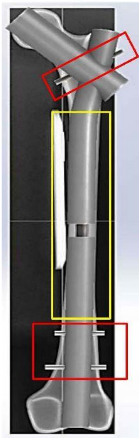
Figure 7-10 Femur and ALFN contact conditions
