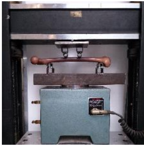
Figure B-4 Four-point bending test setup in the Instron machine
