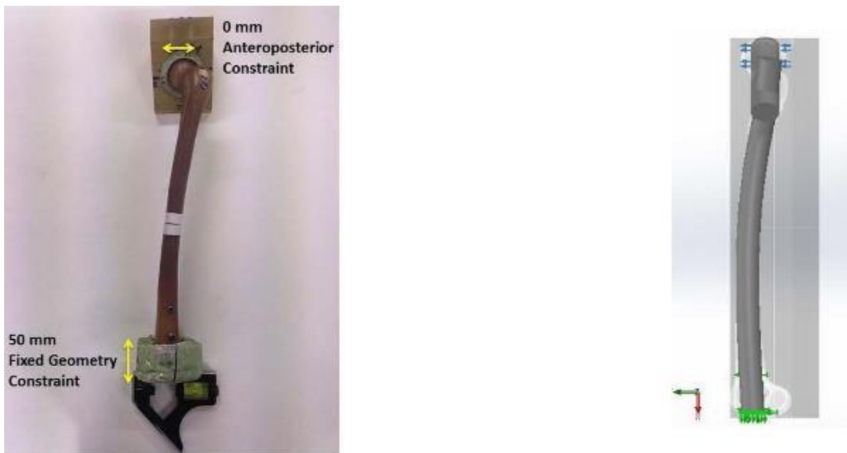
Figure 5-9 Axial compression test boundary condition (left - experimental setup, right – simulated axial compression)
