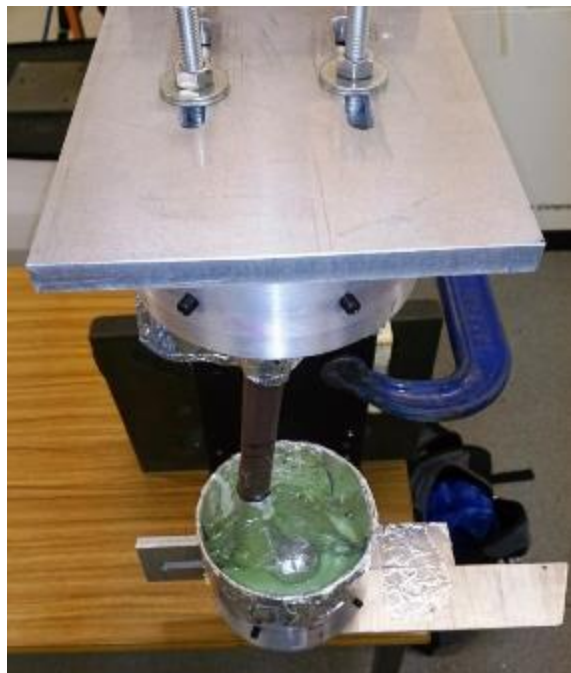
Figure B-7 Femoral head aligned to centre of the proximal cylindrical unit during casting of PMMA mold
