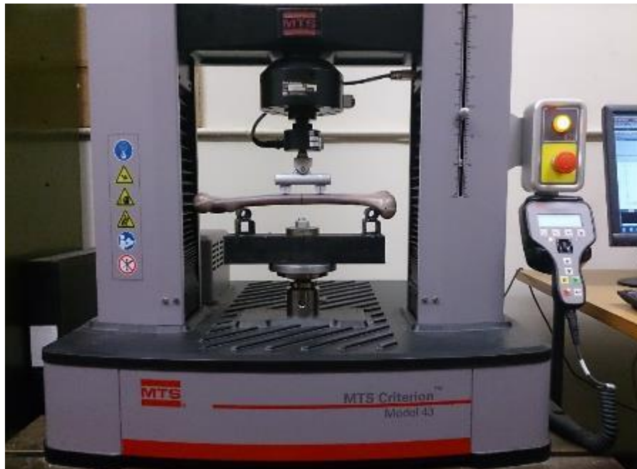
Figure 6-10 Four-point bending test set up using the MTS machine with control femur
