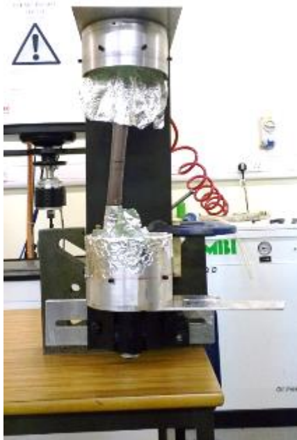
Figure B-8 Alignment of femur during casting of PMMA molds to ensure mechanical axis of femur was coincident with axis of rotation of the jig
