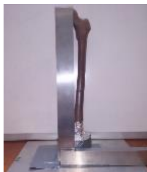
Figure B-3 PMMA split mold at base aligning the femur along the mechanical axis
