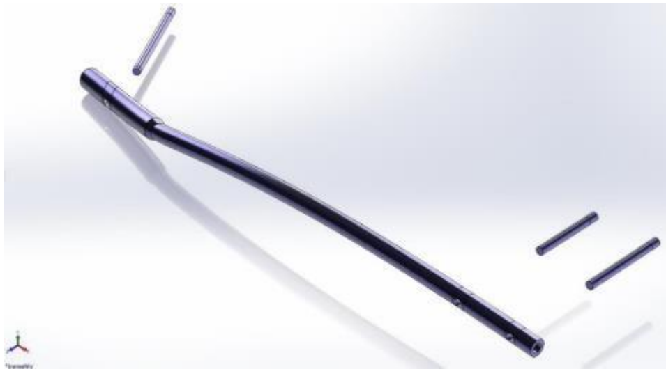
Figure 7-4 Isometric view of CAD models of ALFN, proximal and distal interlocking screws
